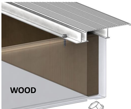
Aludeck System P-6 installed on a Wooden StructureSCREW # 5/30
